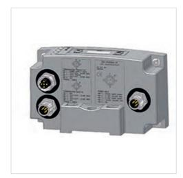
Ambient temperature min./max. -10 ... 50 °C 24 V DC Operational voltage electronics Electronics voltage tolerance -10% / +10% Power consumption electronics 0.08 A 24 V DC Operating voltage, actuators Total current for actuators 4 A IP65 Protection class Number of solenoid coils max. 128 Number of valve positions max. 110
