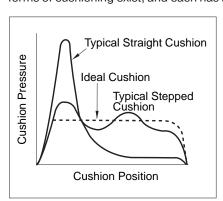
its and advantages. In order to cover the majority of applications, HMI cylinders are supplied with profiled cushioning as standard. Final speed may be adjusted using the cushion screws. The performance of profiled cushioning is indicated on the diagram, and cushion performance for
