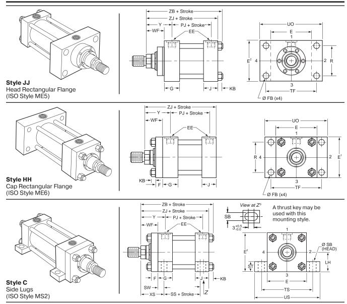
$^{1}$ Head depth increased by 5mm to accommodate port on 25mm and 32mm bore cylinders – see page 5
