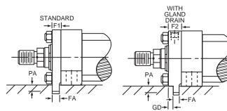
Profile of thrust key extension (with gland drain in retainer) for bore and rod combination 32mm x 22mm.
