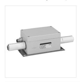
Mounting orientation Any 10 bar Working pressure min./max. 5 ... 50 °C Ambient temperature min./max. Medium temperature min./max. 5 ... 50 °C Medium Compressed air Max. particle size 50 µm Oil content of compressed air 0 ... 1 mg/m<sup>3</sup> 300 mA Max. power consumption \*) Response time 15 ms Precision (% of full scale value) See table below Protection class IP54
